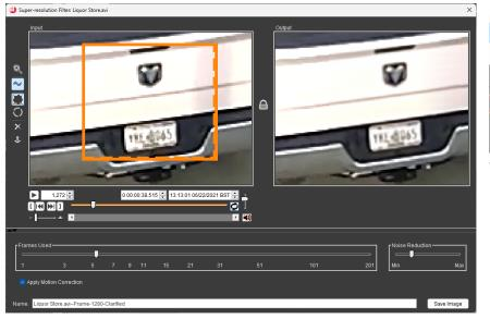
Our Super-resolution filter combines the pixel information across several successive video frames to extract a higher-resolution still image. Unlike simple frame averaging, this algorithm compensates for minor movement between images to minimize blurring while improving the overall definition.
